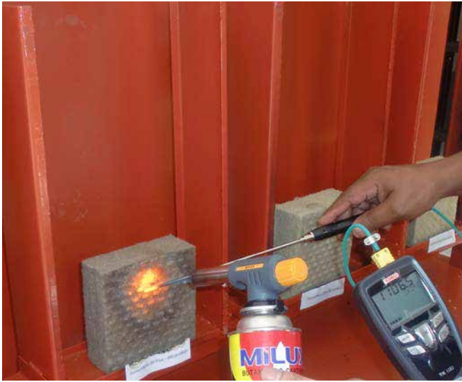
Fire demonstration showing Conlit products withstanding temperature above 1000°C
